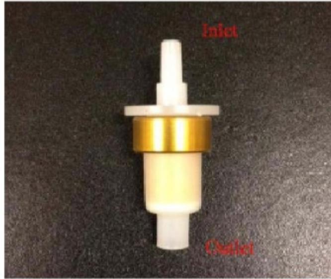
**Figure 6. Carbonyl Sampling Cartridge**
