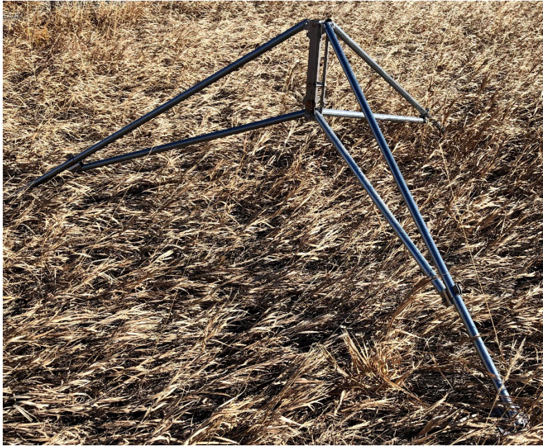
Figure 5. Base of the tripod as erect without center mast
