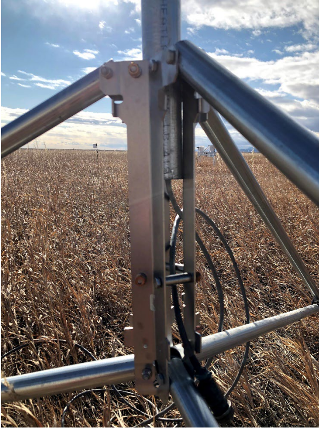
Figure 6. Galvanized plates with bronze nuts at the center of the tripod base
