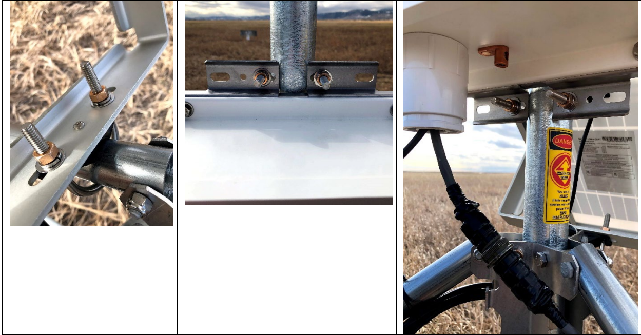
Figure 7. Solar panel mounting hardware (left), Enclosure mounting hardware top (center) and bottom (right)
