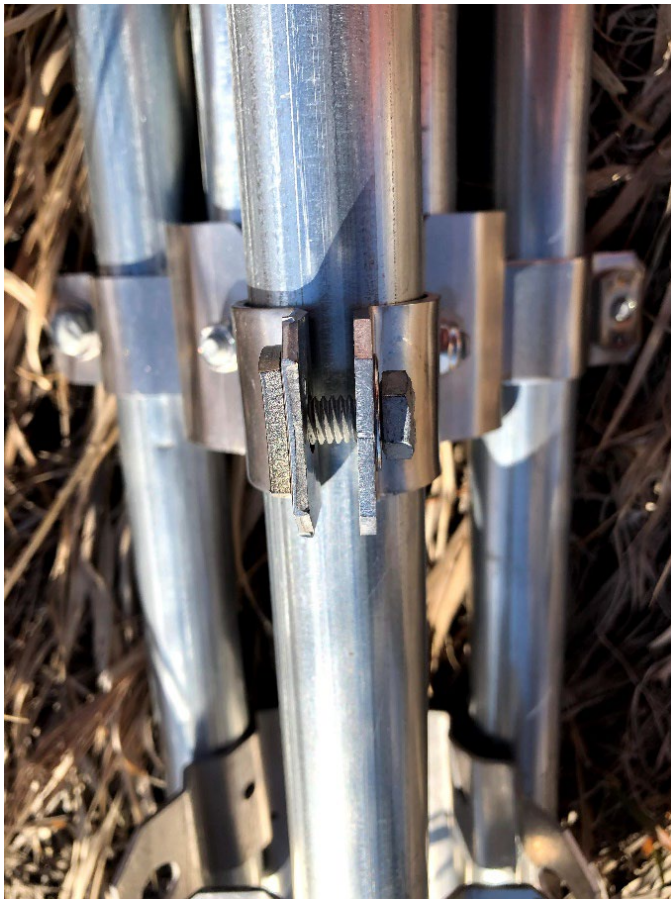
Figure 4. Leg locking clamps with ½ inch bolts
